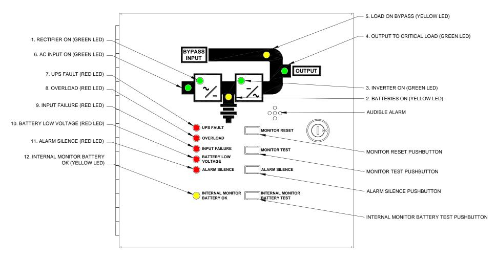
FIGURE 1.1 (INTERNAL POWER SUPPLY / HARDWIRE OPTION)
