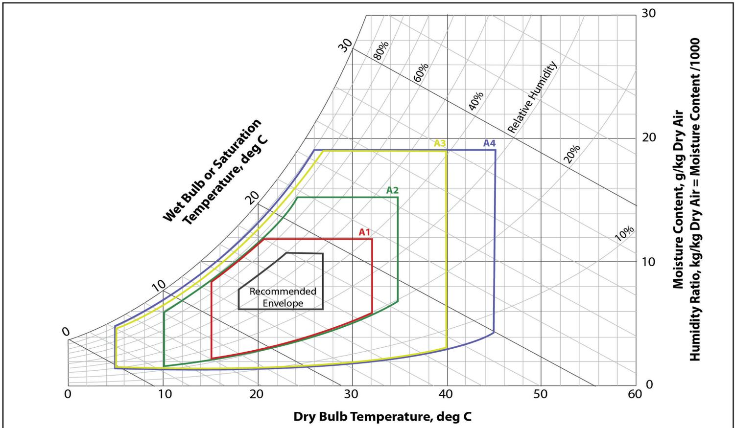
Figure 1: ASHRAE Temperature & Relative Humidity Recommendations for Data Centers
