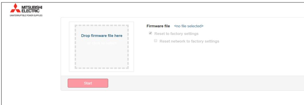
From here you can select the desired firmware package by drag & drop or by clicking the button. Please note that this function is a rescue system, the CS141 will reset all settings except the IP address. All configurations are deleted, and the device is set to startup configuration.
