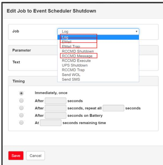
→ **RCCMD Shutdown:** The RCCMD shutdown sends a signal to an RCCMD client. The RCCMD client tells the server to initiate its shutdown sequence.
