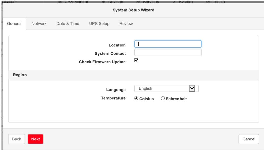
The Setup Wizard helps to set up the basic CS141 configuration and has the following tabs.
