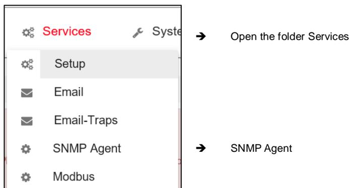
The CS141 can fully be integrated into a network with SNMP monitoring. The built-in SNMP agent regulates both receiving and sending corresponding requests and supports SNMP V2 and SNMP V3.
