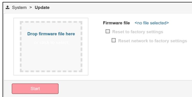
Drag the update file directly to the provided window. Selecting Start will trigger the update process.
