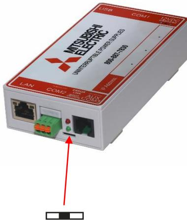
In factory default setting (the slide switch is in the center position) the CS141 is in configuration mode.
