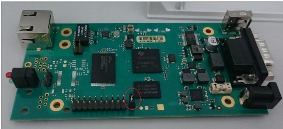
If the jumper is set and the adapter boots the CS141 will run this version as a rescue system based on the last firmware version.
