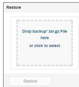
Use drag & drop to place the packed file into the box or left click on the box to open a file browser and double-click on the desired backup file. With Restore, the recovery process will be triggered. During the recovery process the CS141 unpacks the file and automatically takes over as a current configuration. After completing the process, you will automatically be logged out and have to re-login with credentials according to the backup.
