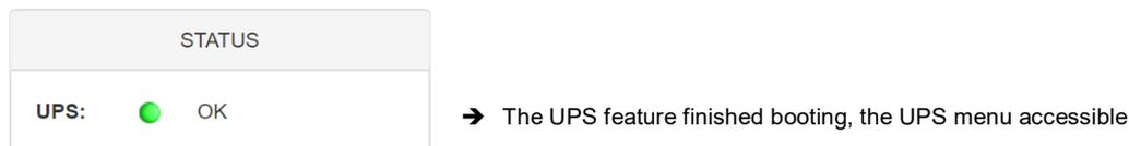
Please note that only a dummy UPS monitor without function has been started at this point, even if a UPS is apparently connected and in operation.
