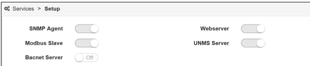
To enable or disable the according service, use the buttons. Switch to the right means the service is enabled, switch to the left means the service is disabled.
