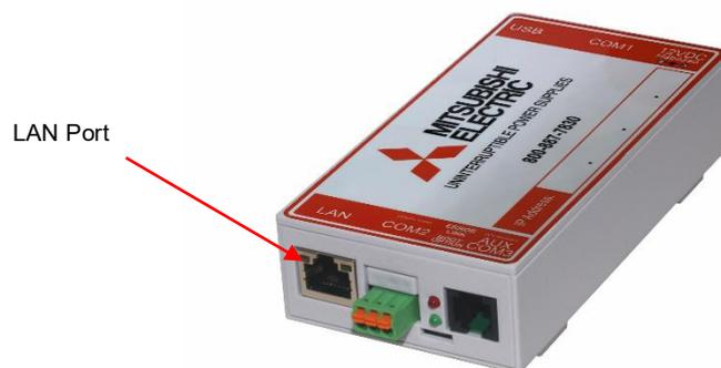
The CS141 complies with RFC1628 standards. If required the MIB can be provided by contact Mitsubishi Electric Power Products, Inc UPS support.
