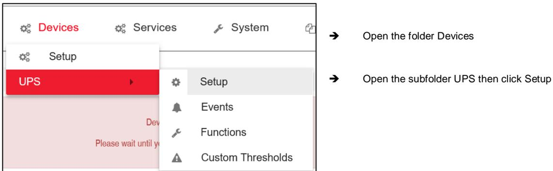
Proceed to submenu UPS and click on Setup to enter the basic UPS configuration menu.
