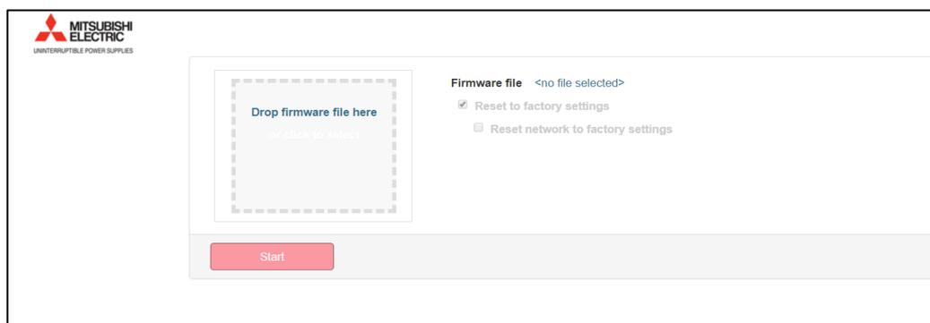
Select the check box for Reset to Factory Settings and hit next. This will delete the basic device configuration but keep the network settings.
