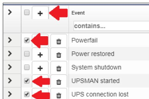
To speed up the process select the events that should receive the same job with the check boxes, then click on the +. By doing so the same jobs are created inside the selected events.
