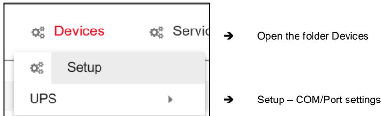
To start configuration, go to Devices and press Setup.
