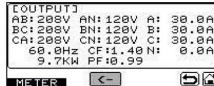
**▲ Figure 14 Measurement During Battery Operation**
