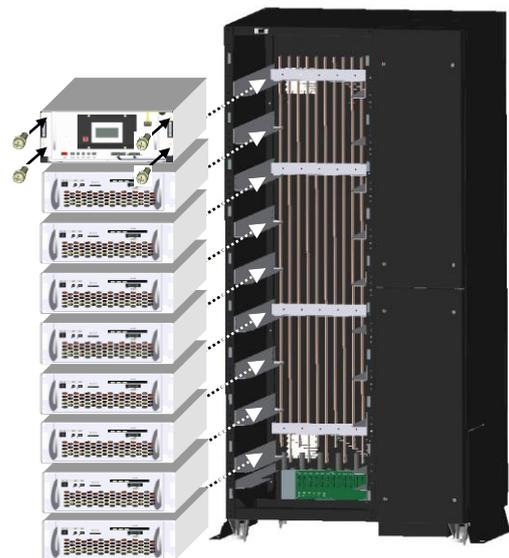
3. Fastening four (4) screws in each module
