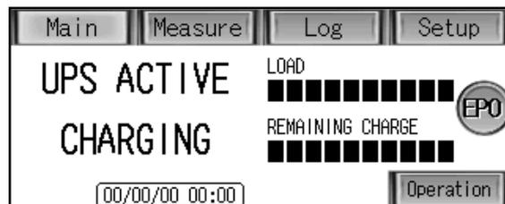
The Liquid Crystal Display (LCD) touch panel indicates how the power is being supplied to the load, measured values, data records and error messages. The LCD panel has a back-light which facilitates viewing in different ambient lighting conditions. The LCD will automatically clear and turn off if the screen is not activated within a 3 minute period. The LCD is turned back on by touching the screen.
